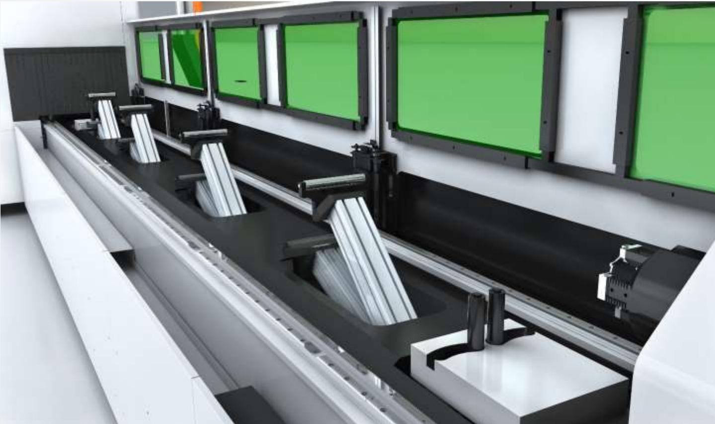
**Rolling support, avoid tube sagging while cutting small tube and heavy tube;**
