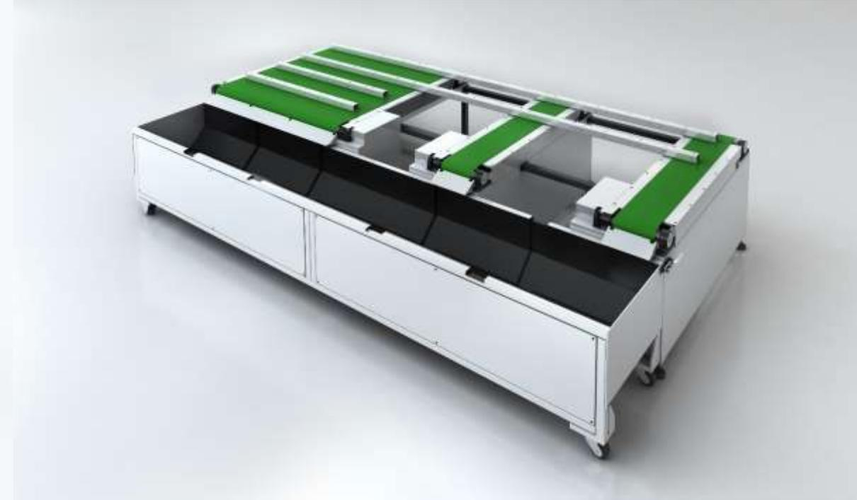
**Automatic feeding system, bundle tubes can be intelligently sorted and single tube feeding is completed in one go;
